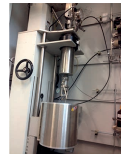
Typical propoxylation reactor for the synthesis of polyethers
